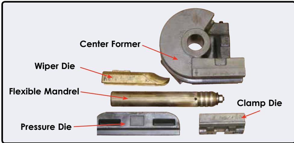
Ercolina mandrel systems incorporate five (5) individual tooling components to effectively support the profile during bending process. These components; **Center former**, **pressure die**, **clamp die**, **wiper die** and **flexible mandrel** are specific to material type and dimension.
