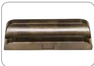
**Pressure Die:** Maintains constant pressure on tube at tangent where the bend occurs, providing reactionary force to make the bend. Length of the pressure die depends on the degree of bend (DOB) of part being bent and the machine design.
