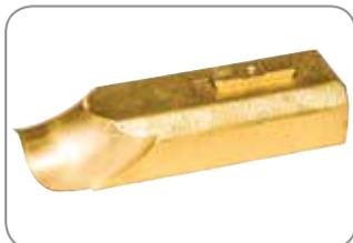
**Wiper Die:** Manufactured to match center former radius. Mounts into the groove of the center former with tip positioned near tangent point of bend. Primary function is to prevent wrinkling on the inside radius of the tube. Wiper dies are typically manufactured from AMPCO® bronze.
