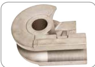
**Center Former/Bend Die:** The primary tool which determines bend radius. Manufactured from tool steel or alloy steel and heat treated depending on requirements. Clamp face is serrated to assist grip strength.
